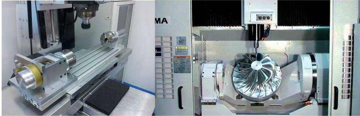
(a) (b) Figure 2 – Axis configurations; (a) 4-axis CNC mill[9] (b) 5-axis CNC mill[10]
